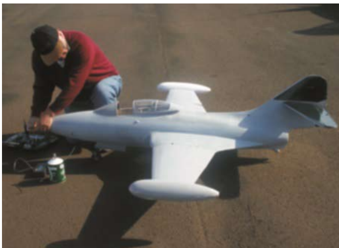
Folding wing Panther powered by Dad's home built GT200 gas turbine
