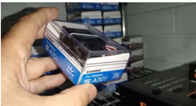
Torque 8.5kg/cm on 6 volts - 9 on 7.4
