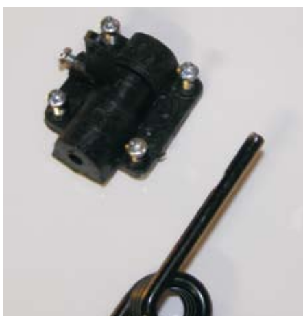
Make your own access to service the nose gear steering arm.
