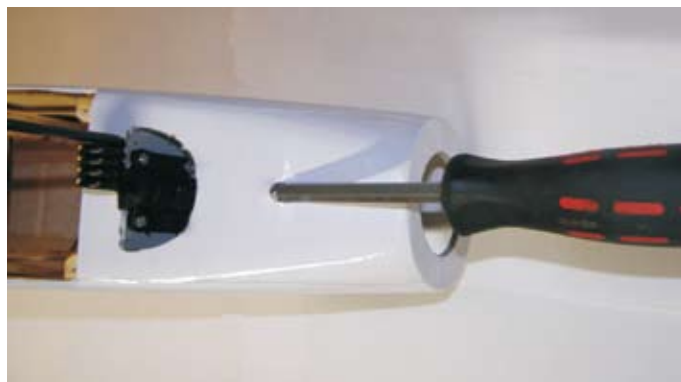
Make your own access to service the nose gear steering arm.
