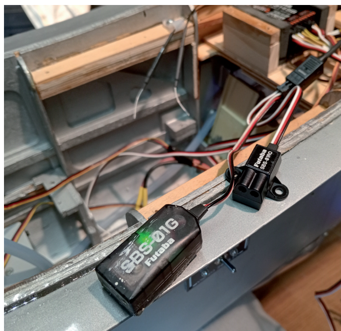
GPS for ground speed, Opto RPM and water temperature telemetry sensors
