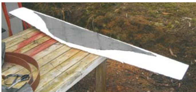
Wing skins are 3mm balsa with carbon fibre sandwiched in between the foam core. A 3/4 span full depth spar was added before vacuum bagging the entire wing.
