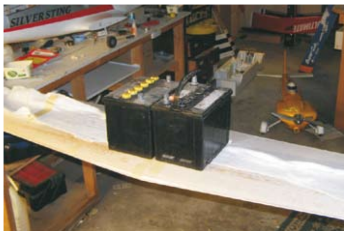
Very glad not to hear a crack or a creak with this 37 kg static weight test.
