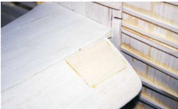
Hinging and control horns and full depth ply spars.
