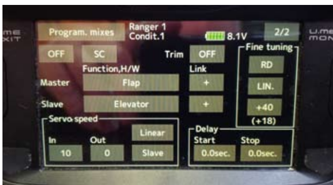
Setting the Flap Function as the master is another way
