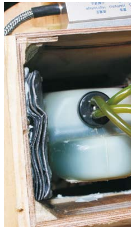
Lead glued with silastic
