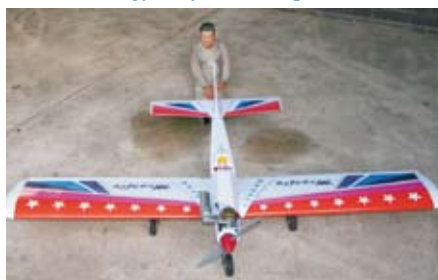
Sighting everything from the rear makes it easier to correctly align all of the control surfaces.
