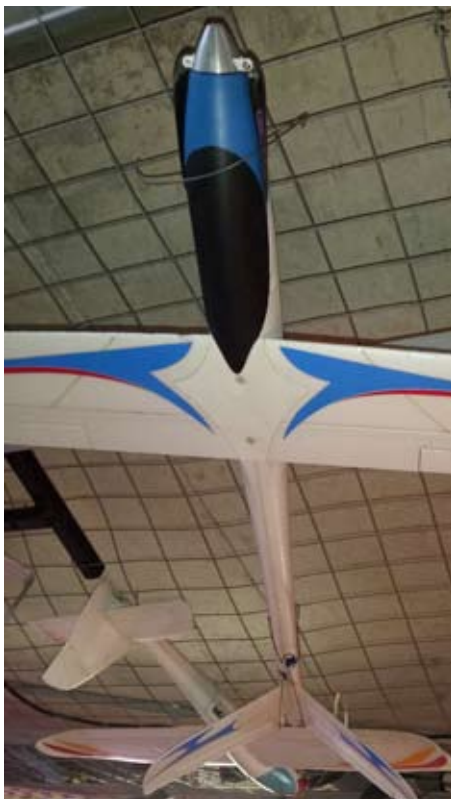
Multiplex Blizzard R3106GF Antenna pokes outside underneath the wing
