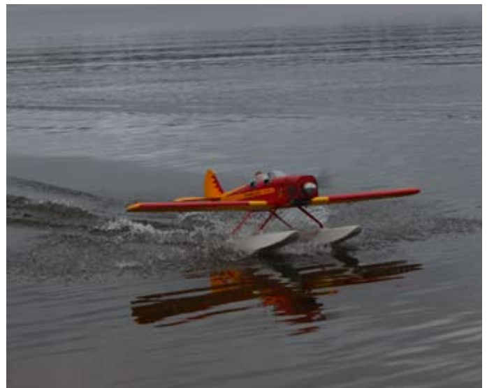
Raising the nose to keep tips out of the water
