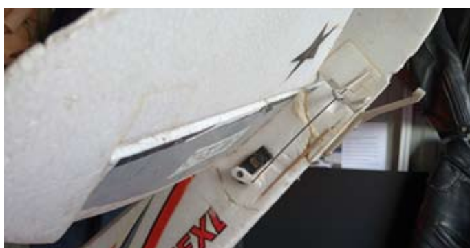
Hitec digital servo replaced with a small JR
