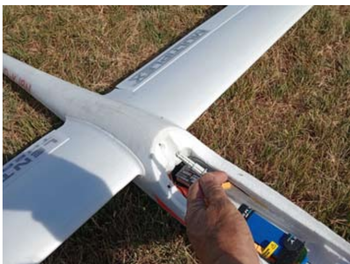
Push the retaining plug in
