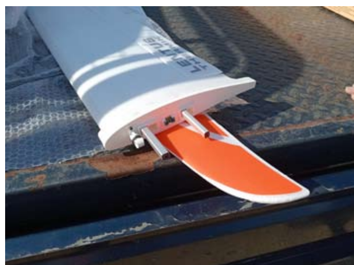
Slide each wing panel into place
