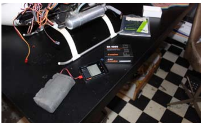
Battery pack wrapped in Dubro latex
