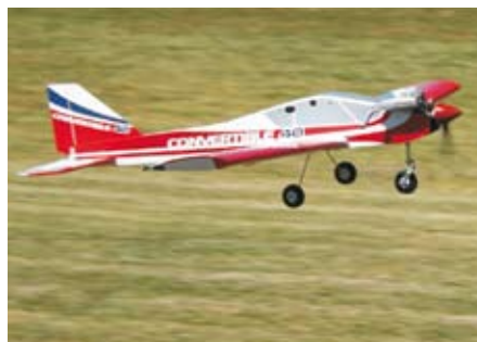
Phoenix Convertaplane flown at Sandown 2016, High wing, low wing or this configuration the only difference was elevator trim
