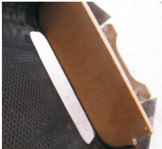
A Lite Ply baffle in the belly pan directs the hotter battery cooling air exhaust out through a slot in the pan
