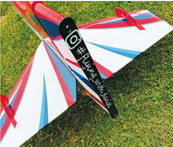
Thick trailing edge on Dan Wheeler's model softens control response around neutral. Dan recently moved up into in F3a class
