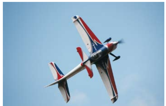
Current generation FMS Olympus foamy much easier. Control surface throws were Aileron 12mm each way, Elev 16mm, Rudder 15mm. Measured at the tip or top. Excellent model, until it just flew away on DSM
