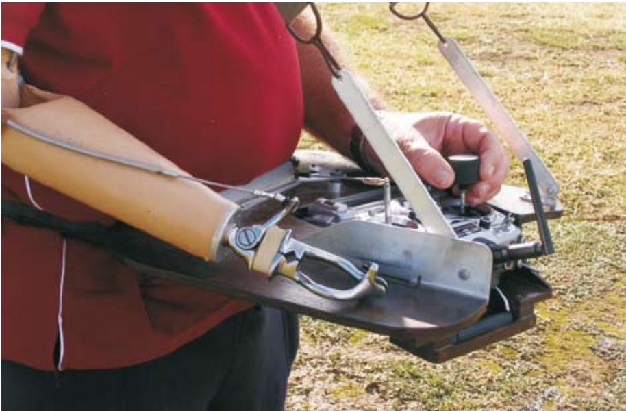
John Payne flying single stick at an Australian Masters. Knob on top is rudder, throttle cable on right hand side
