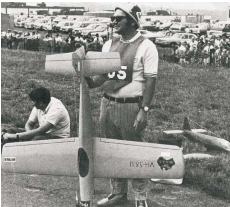
Brian Green and Dragon Fli at Doylestown USA 1971 OS 61 Goldhead, rear induction drum valve loop scavenged. 660sq in wing, weight 8lb 11 oz (3.94kg)
