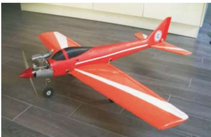
1980s MK Champion 60 fixed gear plastic fuselage foam wing ARF
