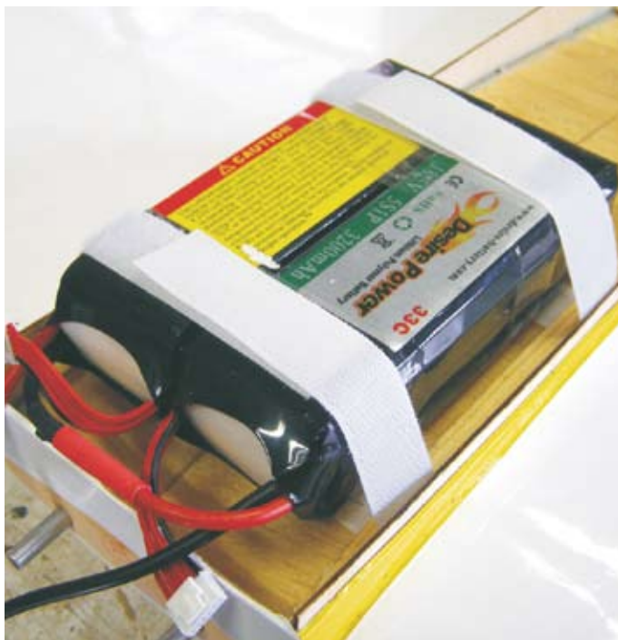
Battery held in place. Simple and effective
