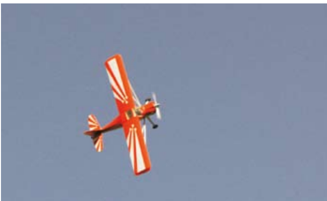
Heaps of opposite aileron needed for knife edge
