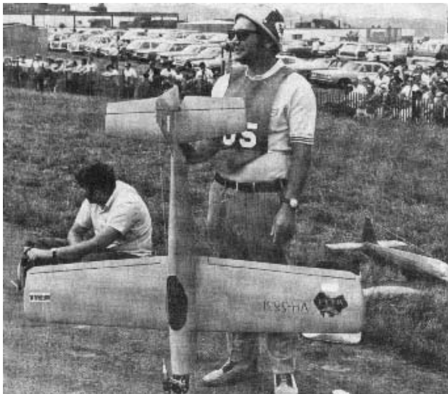
The first ever Australian entry at an aerobatic World Championships, the 7th in 1971. Our Author with his Dragonfli, OS 61 loop scavenged two stroke engine, 11x7 prop, Multicon electric retracts and Kraft six channel 27MhZ radio.
