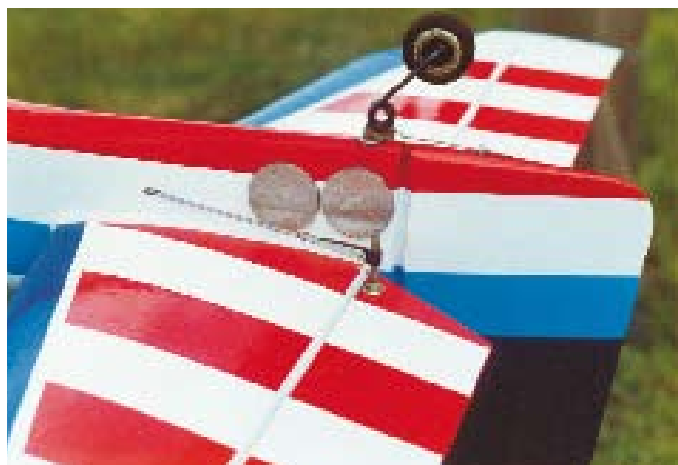
Just one way to move the CG back. International competitor at the Wangaratta World Championships 1991. They are Aussie 50C coins. For a CG further back would you use a dollar note?
