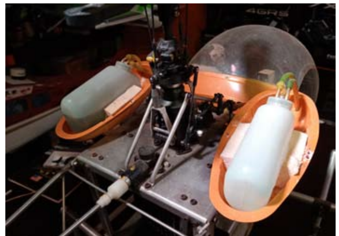
Sullivan slant oval fuel tanks plumbed in series
