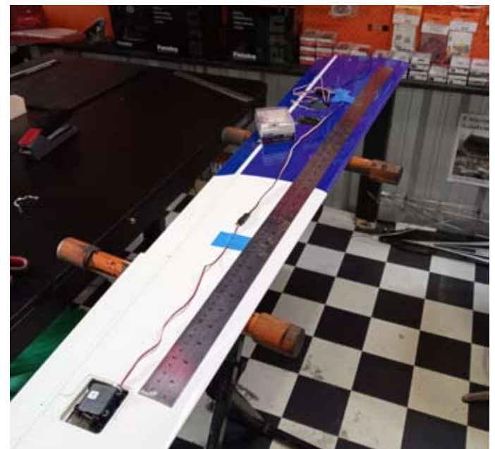
S3173 metal gear ball race glider wing servo for my first all SBus 2 setup
