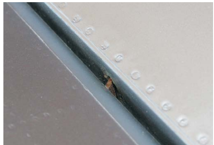
Beauty isn't skin deep. A foam trailing edge to accept hinges was just not up to it. Replace with fibreglass circuit board material
