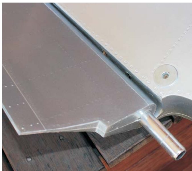
Large flaps on most Mustangs usually does not produce much pitch change when lowered
