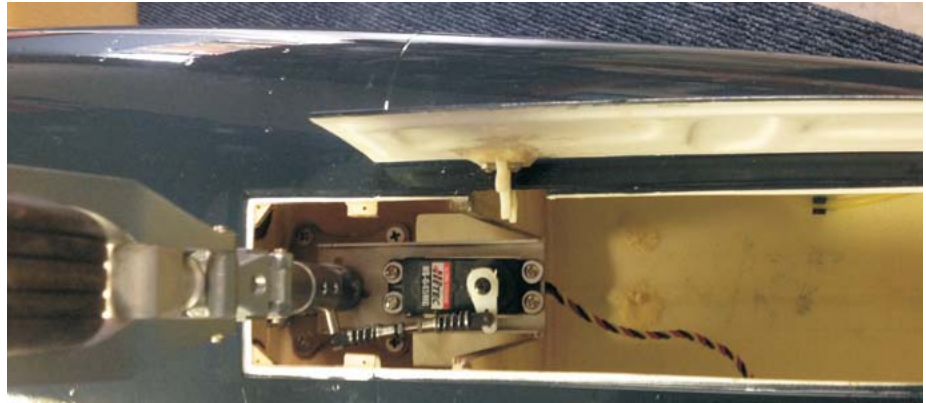
Nose gear steering on rudder channel. Rudder is mixed through free mixer. Steering servo isolated when gear selected up prevents servo moving and pressing stalling against now immovable steering arm
