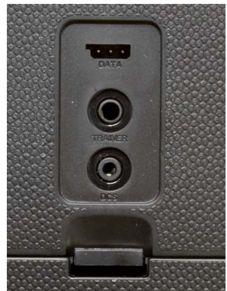
Centrally located data, trainer and DCS (supplementary power output) ports, battery bay hatch
