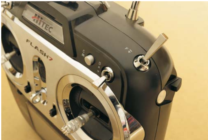
Right shoulder features a momentary push button, two position switch, momentary switch and a slider
