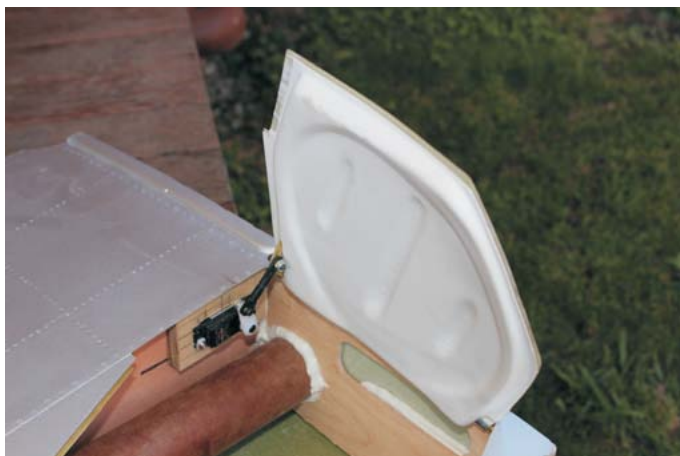
Gear doors operate through an onboard sequencer. This can also be tasked to a computer radio with free mixers and delay timers
