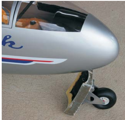
Nose gear dolly (by Rowdy Matthews) is released after takeoff
