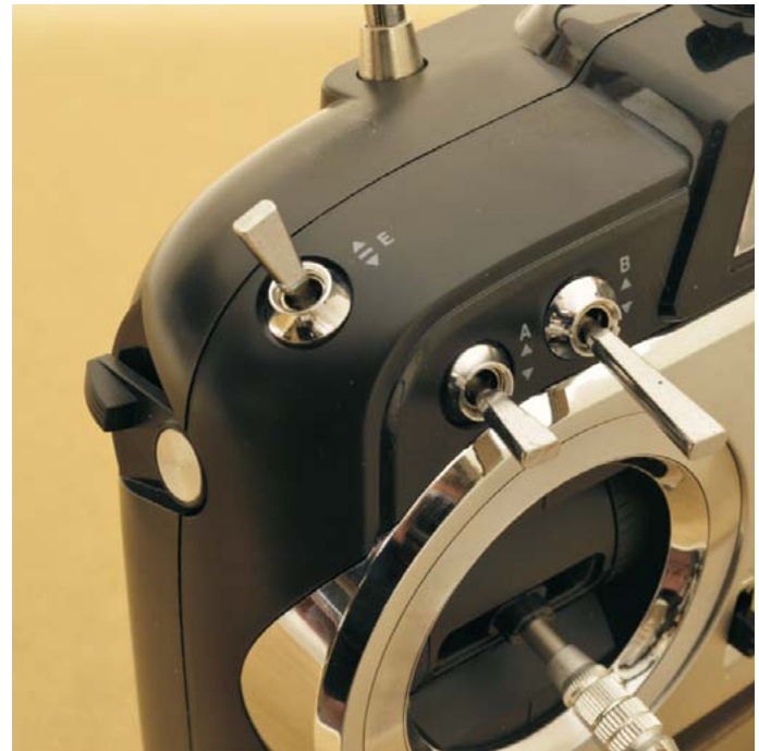
Left shoulder features a slider, a three position switch and two a two position switch
