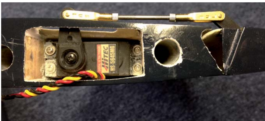
Tailplane halves are similar to the rudder and call for a mini size servo. I managed to squeeze a standard size unit in each
