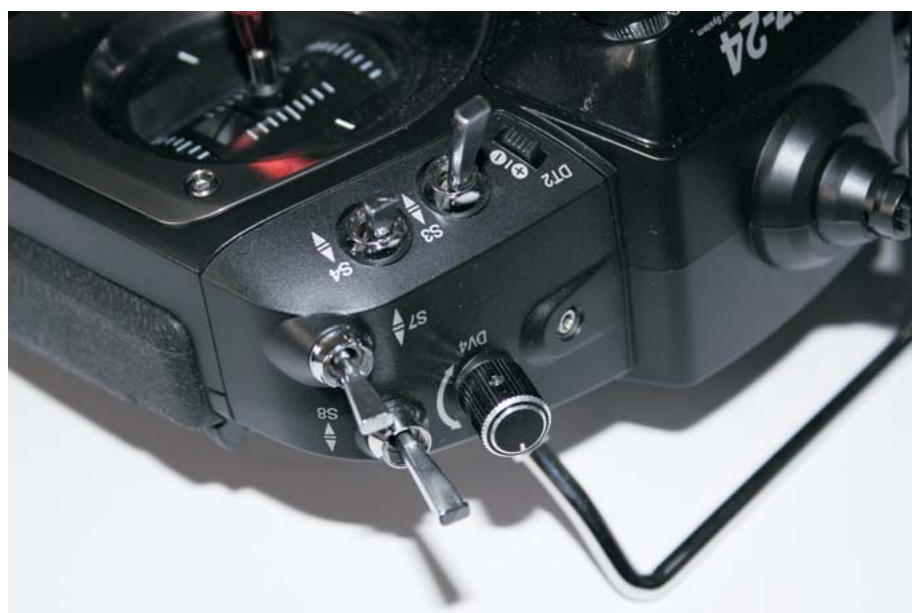
Of the four three position switches, two have a toggle
