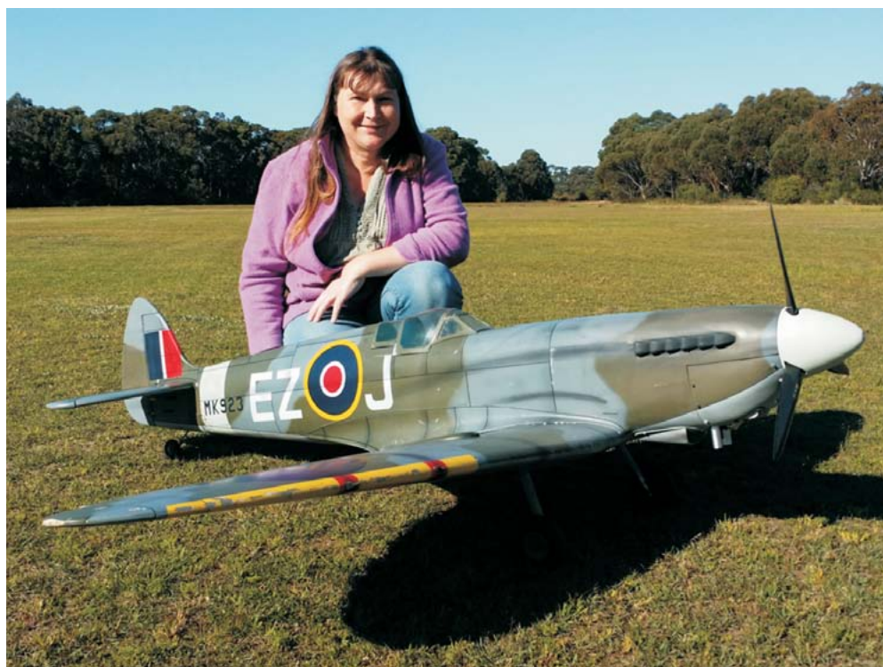
Jaz Cooper and the 1/5th scale Pica Spitfire. Pica kitted the original Dave Platt design, which was powered by an OS 90 glo engine
