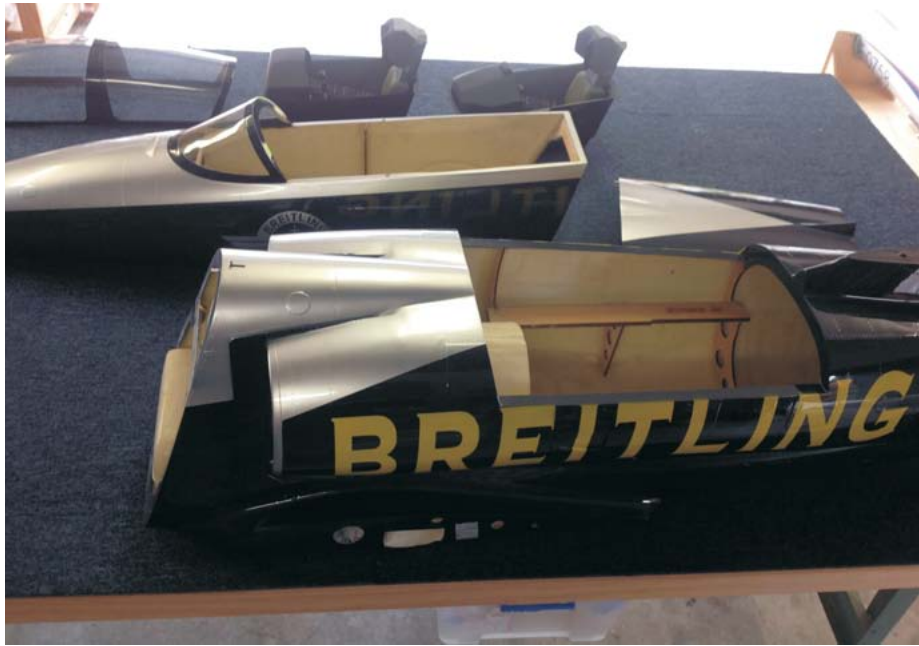
Two cockpit tubs take up a fair bit of room and the rear is a drop fit to assist with monitoring the engine on start up
